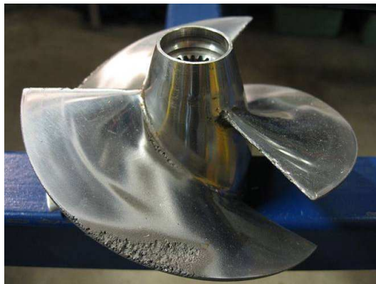
Figure 1.1: Cavitation damage on a propeller blade 1 .
